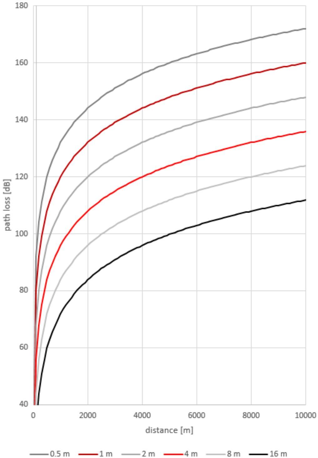
Figure 11: Path losses for different antenna heights
