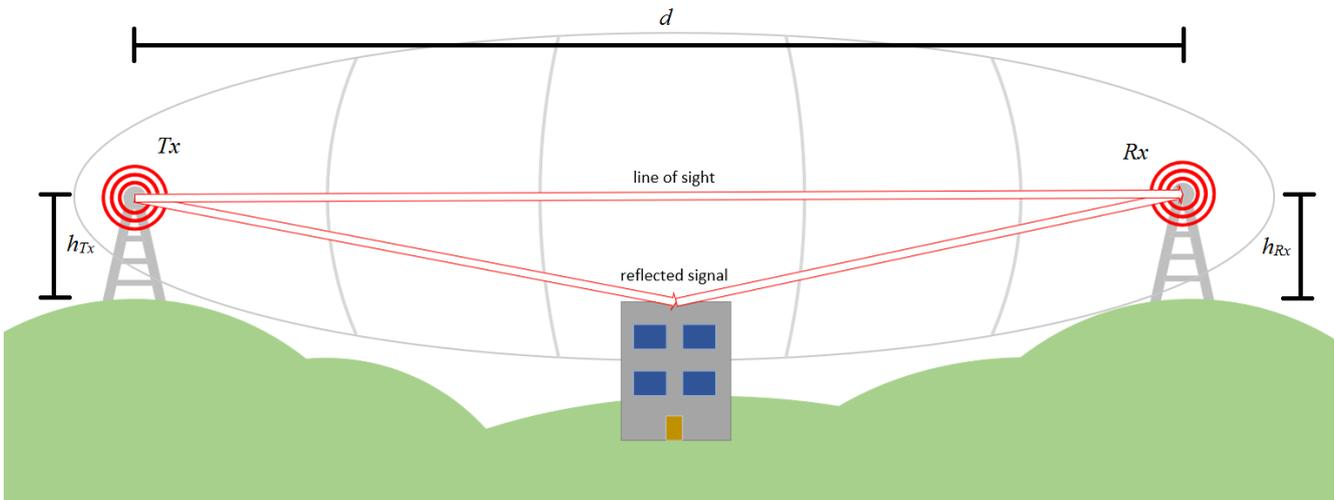
Figure 10: Two ray ground model
