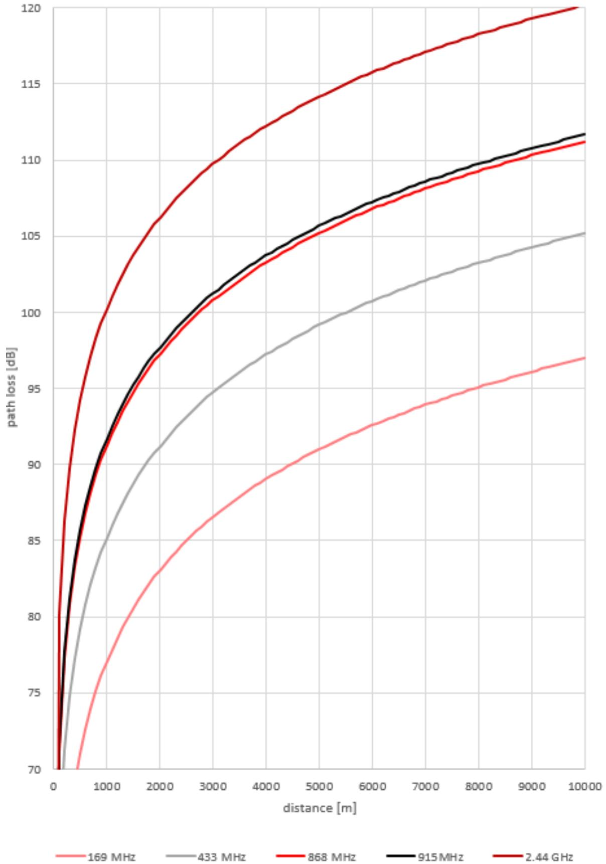
Figure 9: Path losses for different frequencies
